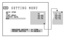
**4** Press the (MEASUREMENT SWITCH), and the cursor moves to the next item(DATE/TIME).
