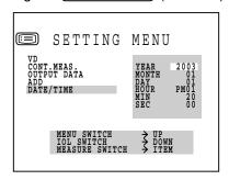
**4** Press the (MEASUREMENT SWITCH), and the cursor moves to the next item(D/MM).
