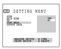
**4** Press the (MEASUREMENT SWITCH), and the cursor moves to the next item(OUTPUT DATA).
