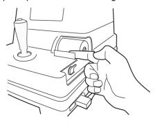
${\it 10}{\it O}$  After making sure that the paper comes out, attach the printer cover.
