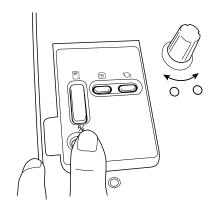
1 Operate the control lever laterally and vertically so as to obtain the target eye in the center of monitor screen.
