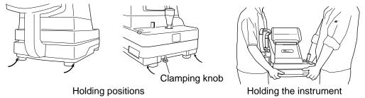
**3** After installation, loosen the clamping knob. Now the main body can be moved.
