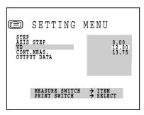
**4** Press the (MEASUREMENT SWITCH), and the cursor moves to the next item(CONT.MEAS.) .
