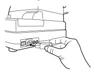
**3** Plug the power cable to a grounded 3-pin AC receptacle.
