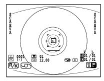
**3** While moving the main body toward the patient, focus the target eye. A vague, reflected luminous point for alignment appears on the cornea.
