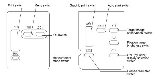
Graphic print switch......Prints out graphically the state of refraction.
