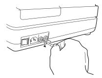
**3** Replace the fuse with the attached one.
