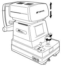
Operating the control lever (for up/down adjustment)
