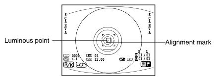
**4** Fine-adjust the main body position in all directions so that the luminous point comes within the alignment mark.
