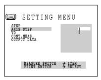
**4** Press the (MEASUREMENT SWITCH), and the cursor moves to the next item(VD).
