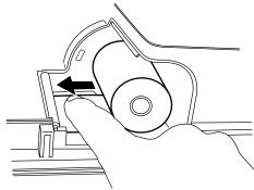
Reset the paper retainer lever to the original upright position.
