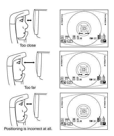
**6** After the alignment bar is displayed, move the main body slowly towards the patient. Measurement is done and the measurement value is displayed on the monitor screen.
