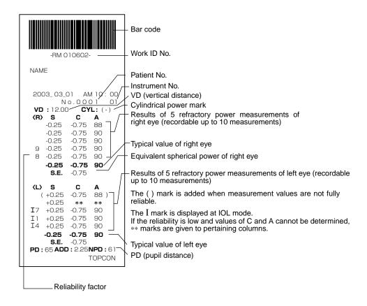
When measurement is done under the IOL mode, a reliability factor is printed out following the I mark.
