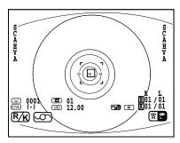
**4** When the luminous point becomes the minimum within the alignment mark, press the (MEASUREMENT SWITCH).
