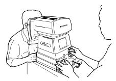
**2** Operate the control lever laterally and vertically to obtain the target eye in the center of monitor screen.
