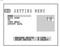
**3** Press the (MEASUREMENT SWITCH), and the cursor moves to the next item(AXIS STEP).
