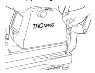
**7** Set the external fixation target (7). Match the connector groove of the external fixation target (7) with the connector of the instrument body and insert it. Secure it firmly so that it does not move.
