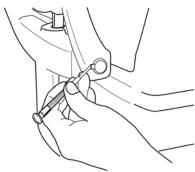
**3** By turning the emergency chinrest knob, insert it into the hole. Make sure of the emergency chinrest knob drops securely into the hole.
