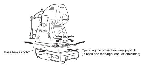
• To move the instrument body up/down, turn the omni-directional joystick right for upward movement, and left for downward movement. The vertical position of the instrument body can be checked with the vertical position mark.
