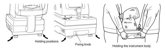
**3** After installing the instrument, fully loosen the fixing knob. The instrument body is freed to move.
