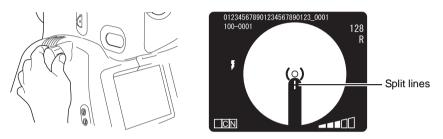
If you cannot align the split lines into one line by operating the focusing knob, change the diopter compensation lens.
