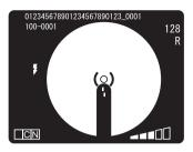
**10** Operate the focusing knob and align the focusing split lines into one line on the color video monitor.
