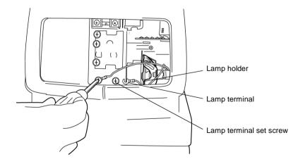
**5** Hold the lamp at the bottom, and pull it out of the lamp holder in a straight direction.
