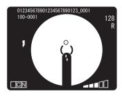
**9** Operate the joystick and move the instrument body to bring the bright spot on the color video monitor into the () scale.
