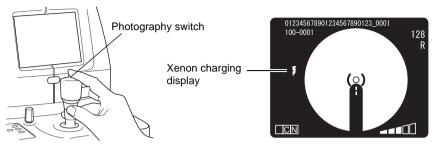
When the xenon charging display flickers on the color video monitor, photography is not possible even by pressing the PHOTOGRAPHY SWITCH.
