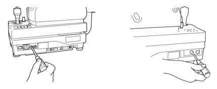
**3** Replace the fuse with a new fuse of the same capacity.
