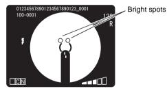
**8** Move the joystick until the two bright spots are changed to one spot on the color video monitor.
