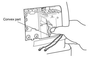
**7** Fasten the lamp terminal securely with the two set screws.
