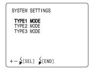
2 Press the <u>FLASH LEVEL SWITCH (+)</u> or <u>FLASH LEVEL SWITCH (-)</u> and select: "TYPE1 MODE" (When taking a picture, recording is done and reviewing is released.)
