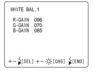
Press the (FLASH LEVEL SWITCH (+)) or (FLASH LEVEL SWITCH (-)) and change each item to the desirable numeral:
