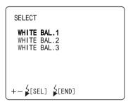
On each of "WHITE BAL. 1" to "WHITE BAL. 3", you can set data. Press the FLASH LEVEL SWITCH (+) or FLASH LEVEL SWITCH (-) and change each item to the desirable numeral: "R-GAIN" (red gain) : The value can be set in the range of "1" ~ "255". "G-GAIN" (green gain) : The value can be set in the range of "1" ~ "255".
