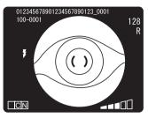
**3** Turn the focusing knob so the anterior segment image is clearly visible on the color video monitor, and press the PHOTOGRAPHY SWITCH.
