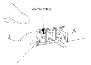
Plug the appropriate approved Power Cord into the Power Cord Inlet on the operator's right-hand side and plug the opposite end into a standard power outlet.
