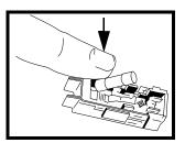
Make sure that the two fuses are inserted so that they are closest to the protruding metal flanges.
