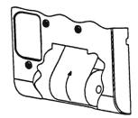
To load a new roll of paper, pull down the **Paper Access Door** (below the Operator LCD Display) using the Finger Tabs on the sides of the door (near the top). Remove the empty paper spool from the paper well.
