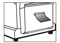
Place the leading edge of the paper onto the metal bar and push it into the unit under the roller bar. The instrument will automatically feed the paper through once you have inserted it far enough.
