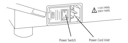
To turn the instrument ON, switch the **Power Switch (O/I)**, adjacent to the power connector, to the ON (I) position. The instrument will perform internal self-diagnostic checks and after approximately 15 seconds, two double beeps will sound and the FDT MAIN MENU will appear on the Operator LCD Display. Refer to the troubleshooting section of this manual if the **FDT MAIN MENU** does not appear.
