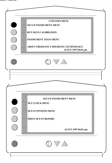
Select **NEXT CHOICE** (3rd Operator Button from the top) to select the clock setting you want to change. (s) **INCREASE** (TOP Operator Button) and (t) **DECREASE** (2nd Operator Button from the top) to change the setting. Select **ACCEPT SETTINGS** (BOTTOM Operator Button) when the **correct CLOCK** settings are displayed. Press the **GREEN Button** twice to return to the **FDT MAIN MENU**.
