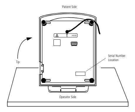
While facing the Patient Side of the FDT instrument, tilt the instrument to plug the **Patient Response Button** connector into the small round connector jack. The jack is located underneath the base of the unit (at the center) and near the patient response button symbol.
