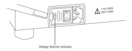
In case you need to change the operating voltage, make sure that the Power Cord is NOT connected and use a flat screwdriver to pry open the Fuse Drawer Cover. Remove the Fuse Carrier/Voltage Selector, by again using a flat screwdriver. Rotate the Fuse Carrier/Voltage Selector so the proper voltage will be visible when the Fuse Drawer Cover is closed. Re-install the Fuse Carrier. Close the Fuse Drawer Cover and check to be sure the proper voltage appears in the Voltage Selection Window.
