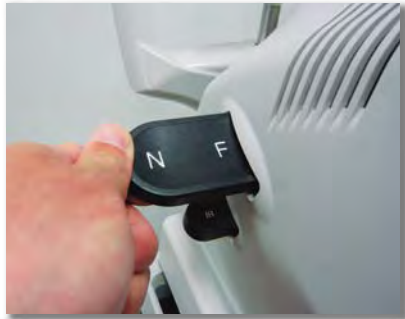
Pull in/out the RF filter selector
